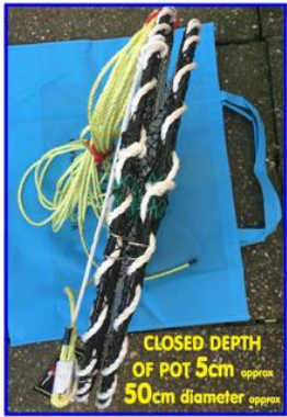
RETAINING CLIPS IN PLACE. NET CLOSED FOR TRANSPORTATION
